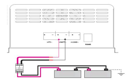
Warning: Short circuit between the positive and negative terminals of the battery and the wires connected to the positive and negative terminals may cause fire or explosion, please be careful Note: Connecting the battery pack must be done with the circuit breaker disconnected
